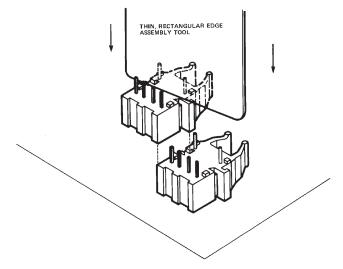
Figure 1. Interlocked (stacked) horizontal packages
