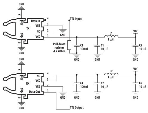
Figure 2. Recommended Transmitter and Receiver Application Circuit
